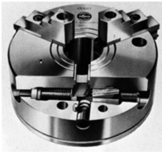
Figure 7.17 Spiral ring chuck with adjustable jaws (photo by Röhm, Sontheim)
