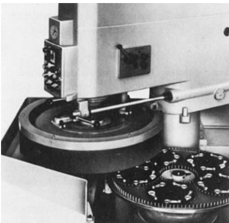
Figure 18.2 Hydraulic two plate-lapping- and precision grinding machine, type ZL 800 H, with planetary driving attachment (photo by Hahn & Kolb, Stuttgart)
