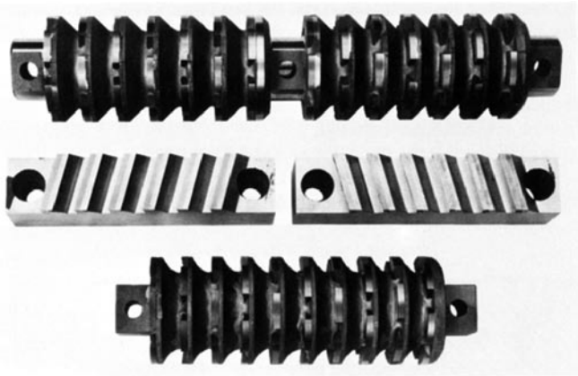
Figure 12.16 Cutting portions with hard soldered cemented carbide tips (photo by Karl Klink, Niefern)
